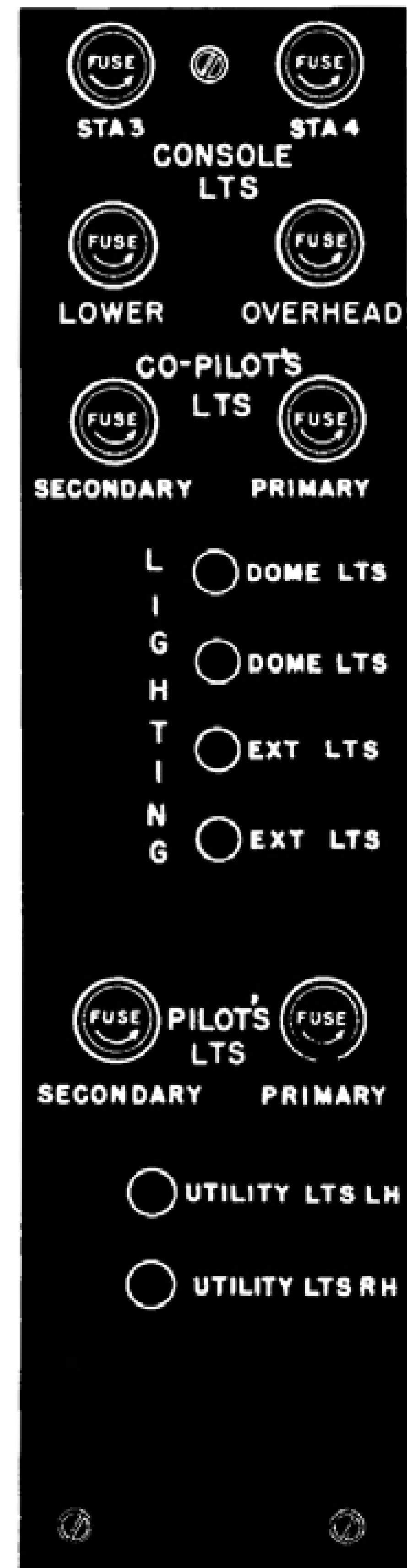
Figure 4-8. Lighting Circuit Breaker Panel
