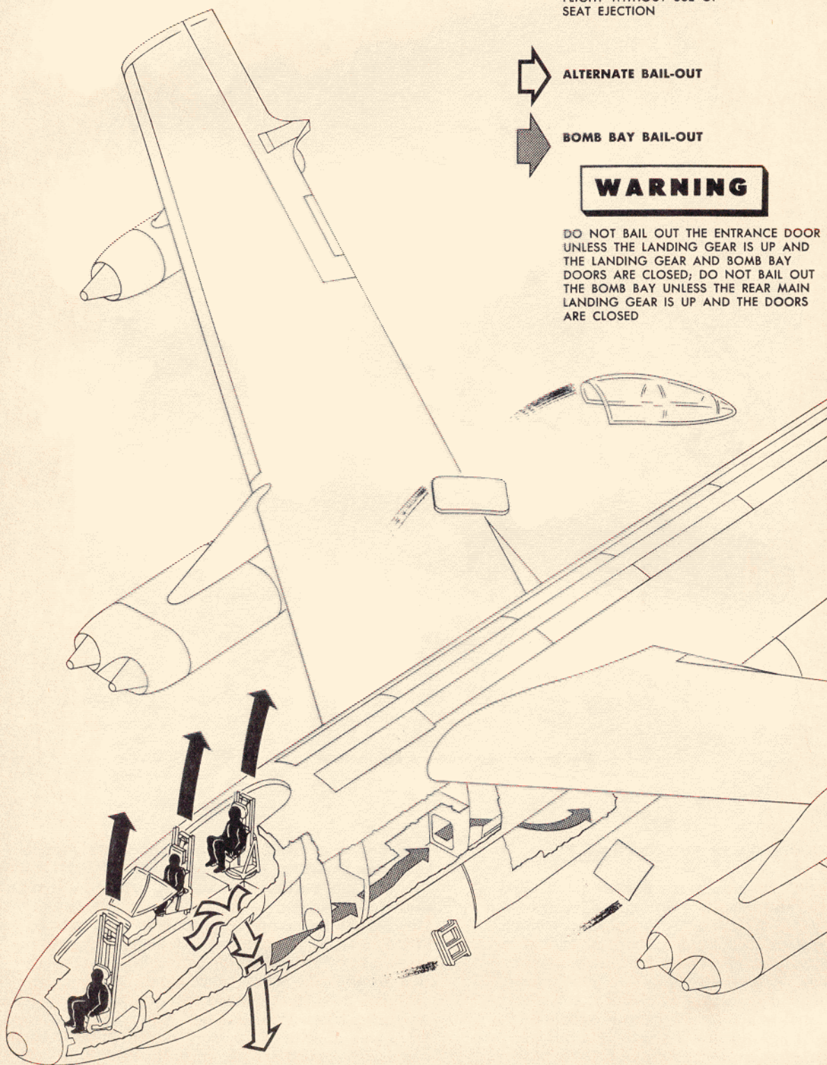
Figure 3-2(Sheet 1 of 2 Sheets). Emergency Exits and Entrances
